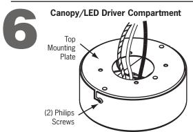
There should not be any excess cable in the ballast compartment. Leave only 6-8" for wiring available.
