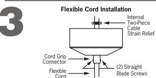
There should not be any excess cable in the ballast compartment. Leave only 6-8" for wiring available.
