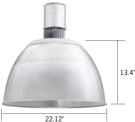
ACL22-(B,P,S) 22" Lexalite™ Clear Acrylic 60° Medium Beam, 0.95 SC
